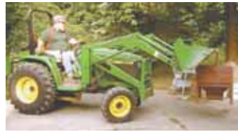
Cement is dumped into a second hopper which loader then moves to trench. There, a trap door on the hopper is manually opened to release concrete.
