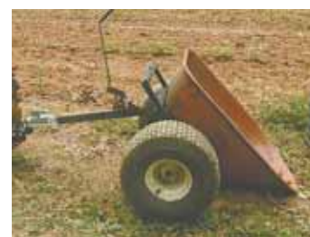
Spring-loaded trip lever is used to dump bucket.
