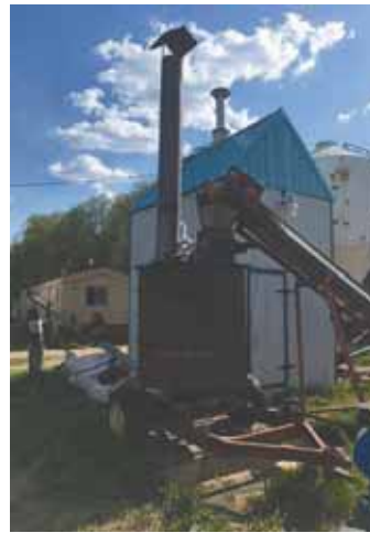
Scrap pipe, an old feed mixer, and a belt conveyor were used to build this continuous-flow biochar machine. Photo at right shows fresh wood chips alongside biochar.
