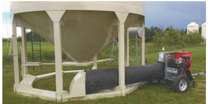
Portable aeration fan is powered by a Vanguard V-Twin gas engine, allowing use in remote locations without electricity.
