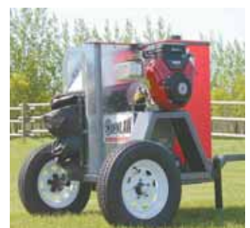
Fan can handle bins from 2,000 to 33,000 bu. for at least 55 hrs. before refueling, depending on static pressure and engine load.
