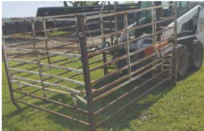
Todd Pieper converted a used pickup stock rack into a handy calf catcher that he moves around with his skid loader.
