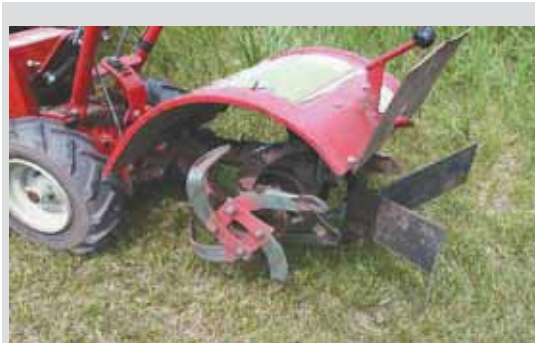
David Sand mounted a V-shaped "hiller" on back of his Troy-Bilt rototiller.
