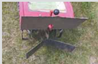
Hiller mounts with 2 bolts in place of rototiller's existing depth control arm.
