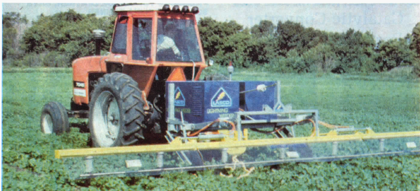
One end of machine's power circuit is electrically in contact with soil through a coulter. Other end of circuit is connected to boom which comes in direct contact with weeds growing taller than crop.
