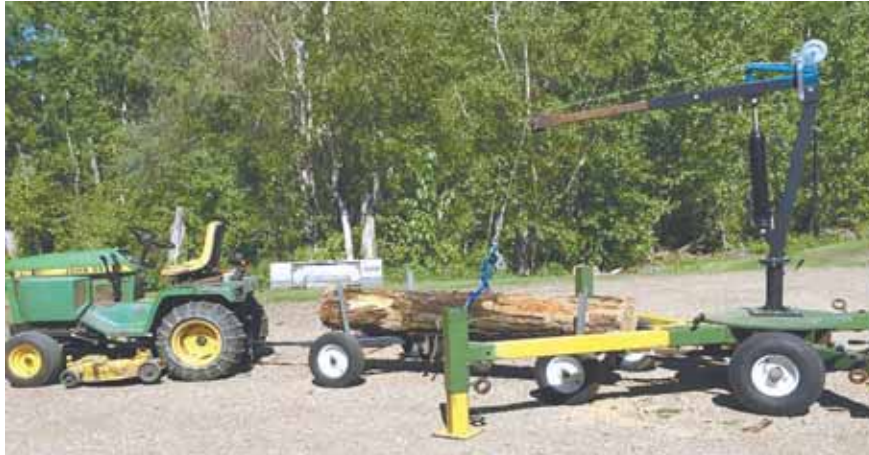
Wes Newman's firewood handling system includes a Deere garden tractor pulling a wagon running gear with uprights, followed by a 2-wheeled swiveling crane with 4 big telescoping outriggers.
