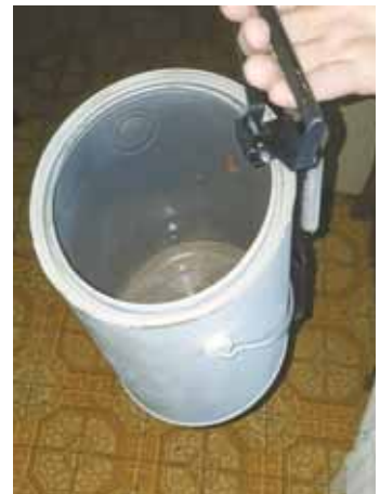
Spring-loaded, 2-piece metal bracket attaches to side of can over original handle.
