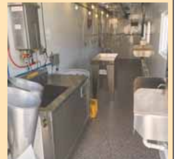
Featherman Pro Set Up includes a picker, scalding, small kill cone stand, and 8 broiler cones (left). Plant In A Box processing plant can handle nearly 500 birds per hour.
