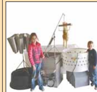
Featherman Pro Set Up includes a picker, scalding, small kill cone stand, and 8 broiler cones (left). Plant In A Box processing plant can handle nearly 500 birds per hour.
