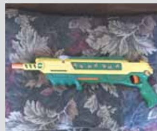
Bug-A-Salt operates on compressed air and comes with a hand grip on front that pulls back to cock the gun.
