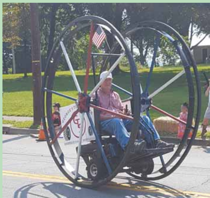
Thomas rides on a Dixon zero-turn riding mower, whose wheels ride on a circular steel band that’s attached to the inside of two 8-ft. dia. metal wheels.
