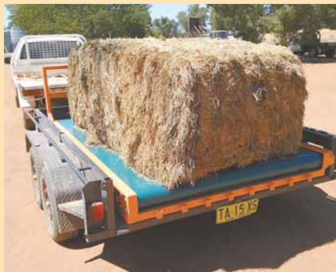
Flakes of square bales slowly drop off back of feeder as belt rotates.
