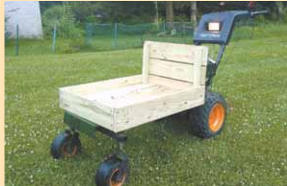
Hanisak bolted a steel frame on in place of snowblower auger, then bolted a 4-ft. long, 2-ft. wide deck onto it. Wheelbarrow is supported by a pair of caster wheels on front.
