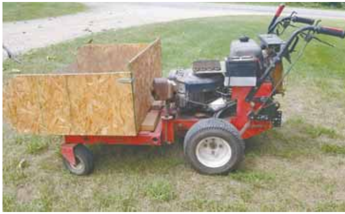
Schmucker lag-bolted a pair of 2 by 10's lengthwise on top of mower frame, then built a plywood box that's attached by a pair of door hinges.
