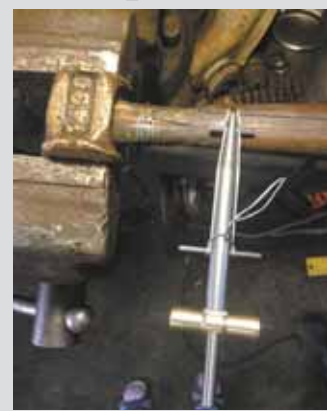
Small size ClampTite is used here to wrap wire around a hammer handle.
