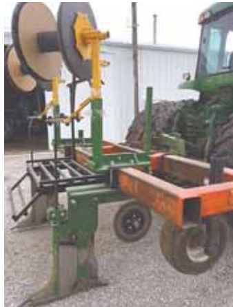
Corner side view of machine shows plow shanks, tape reel holders and operator platform.
