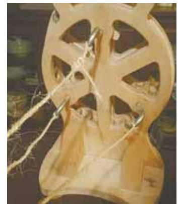
Martin Korson says making the gears was the biggest challenge in building his own rope-making machine (above). Close-up photo shows the wooden gears that drive it.
