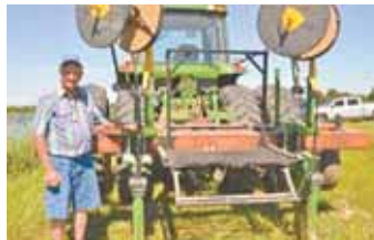
Russ Winter built this machine to install subsurface drip irrigation by himself. "I use it on a 14-acre field that's too small and irregular for a center pivot," he says.
