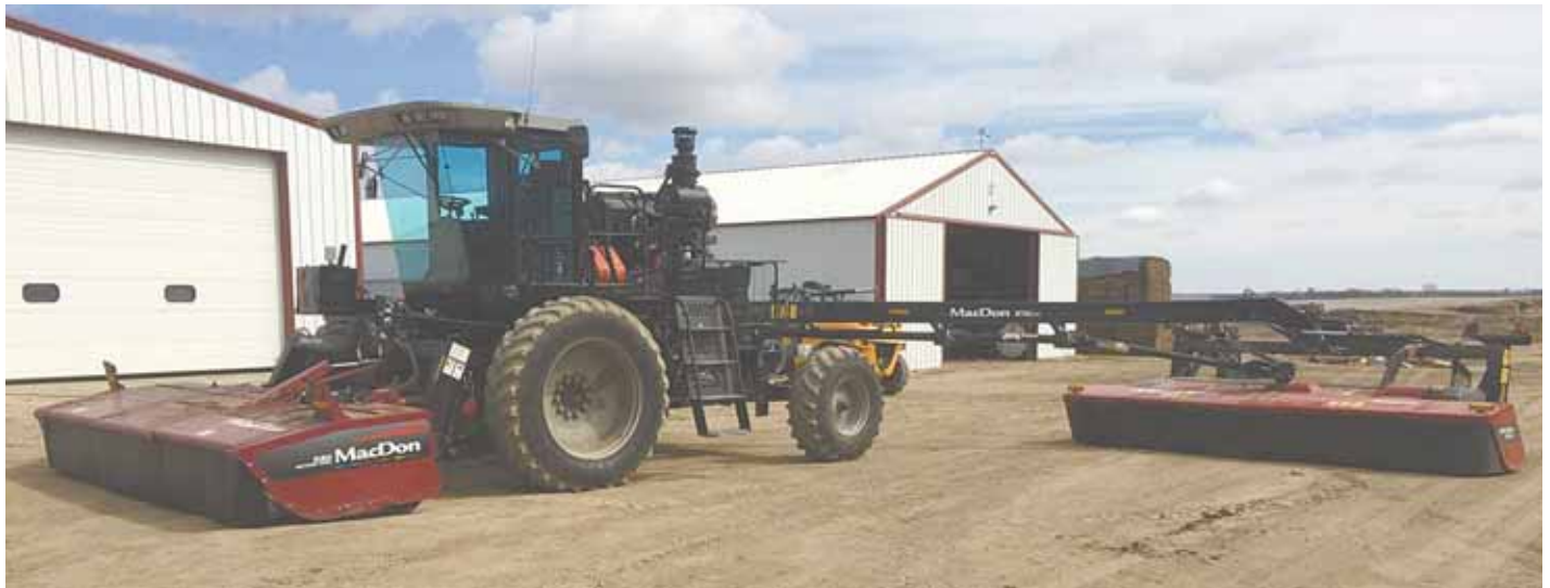
Built out of a 1998 Gleaner R62 combine, Dan Crick's double hay windrowing machine operates two 16-ft. MacDon disc mowers. The entire machine measures 50 ft. long.
