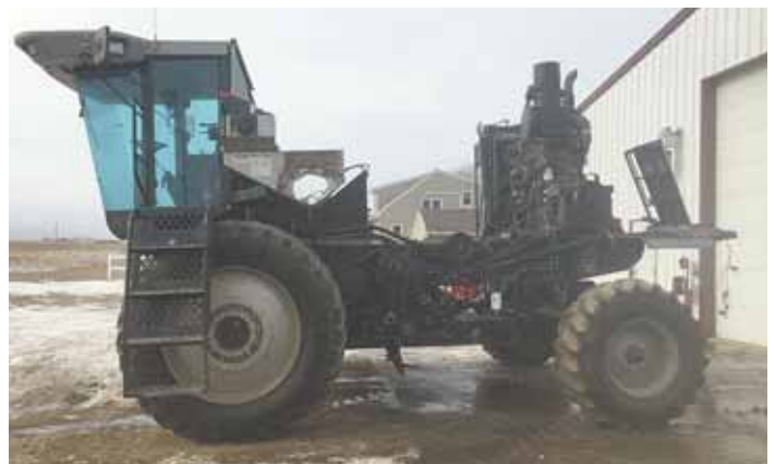
Crick removed all the combine's threshing components, and repositioned the engine. Everything on the combine is belt-driven.
