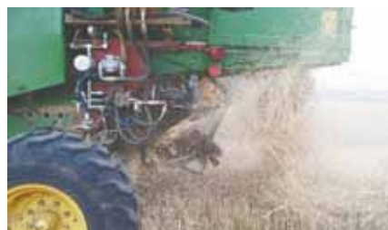
Weed crusher uses 2 sets of discs fitted with 3-in. bolts. One disc of each pair spins while the other is static. Seeds are crushed between discs, then thrown out back of combine along with chaff.
