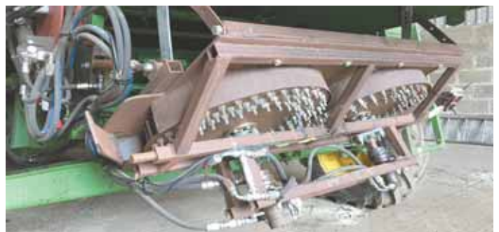
Weed crusher uses 2 sets of discs fitted with 3-in. bolts. One disc of each pair spins while the other is static. Seeds are crushed between discs, then thrown out back of combine along with chaff.
