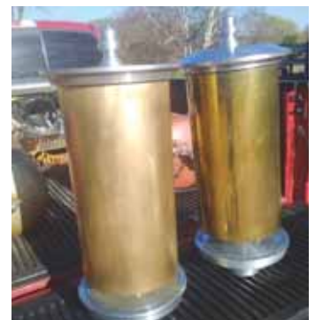
Dave Dam put together these giant brass steam whistles that hook up to a compressed air supply.
