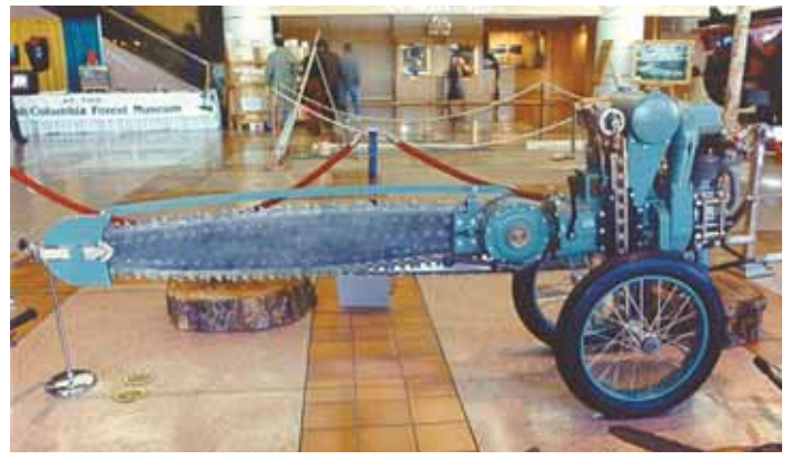
His portable 1933 Dow "low stump" saw rides on wheels and is powered by an Indian Scout motorcycle engine, with a Ford Model A rear end used as a transmission.
