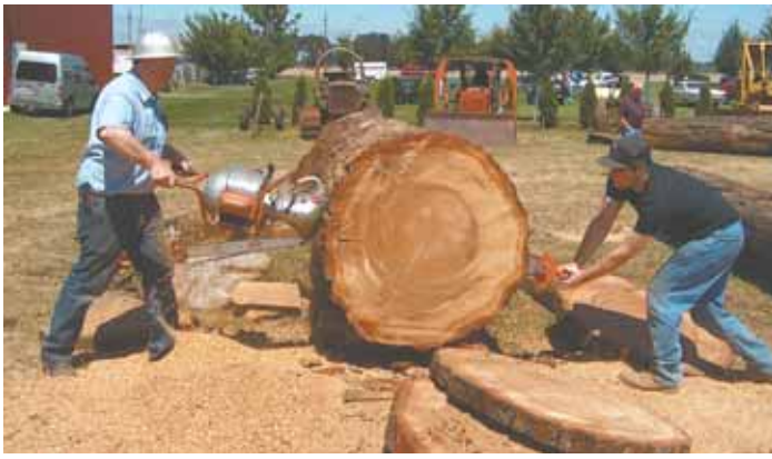
The first chainsaws took 2 men to operate and were expensive, says antique saw collector Marshall Trover.
