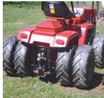
A ball hitch and clevis on back of tractor is used to pull yard equipment. The seat rides on top of a big car spring for a comfortable ride.
