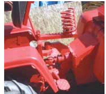
A ball hitch and clevis on back of tractor is used to pull yard equipment. The seat rides on top of a big car spring for a comfortable ride.
