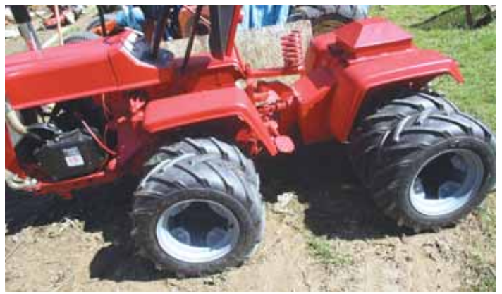
“It's modeled after a real IH articulated tractor,” says Phil Murphy about the 8-WD articulated garden tractor he built out of 2 Cub rear ends. It rides on dual 24-in. tires.
