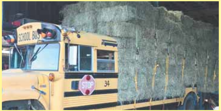
John Rouse converted an IH schoolbus into this self-propelled bale hauler. Bus is loaded by hand, with the bales strapped down to eye bolts welded on bus frame.
