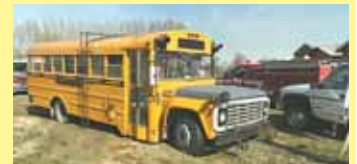
A ladder on one side of bus provides easy access to top of bus for filling tanks.
