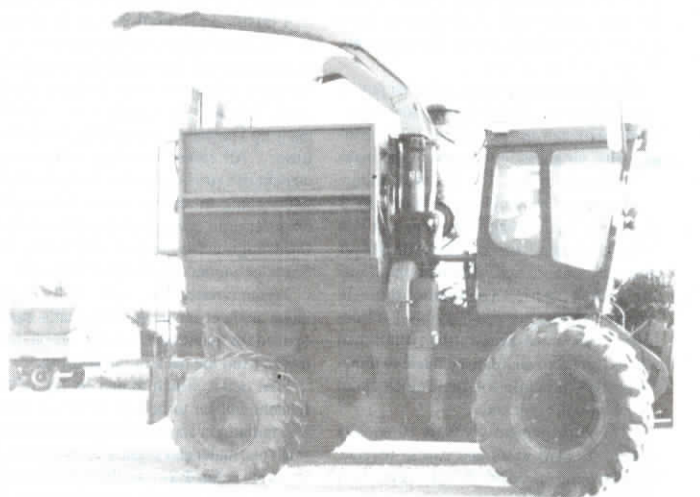
The 8-ft. wide, 4-ft. high, 6-ft. long hopper mounts on a Deere 5460 forage harvester.
