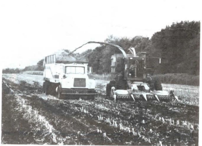
Morgan can switch between two spouts - one that blows into a rear hopper and one that blows into a vehicle alongside.
