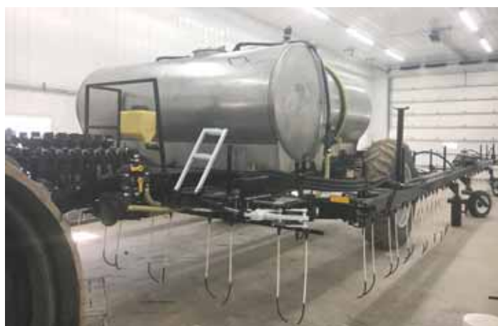
Andy Mulvihill with his brother, Tony, and father, Tim, built this liquid applicator that lets them side dress liquid nitrogen and apply herbicide in one pass.
