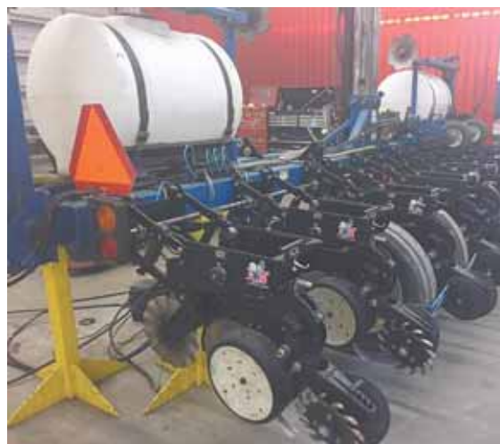
The folks at Kearney Planters say farmers can save money with custom-built planters designed for precision agriculture. Photo shows a Kinze 3500 being converted from a 15-row, 15-in. planter to a 16-row with 8 sets of 7 1/2-in. twin rows.
