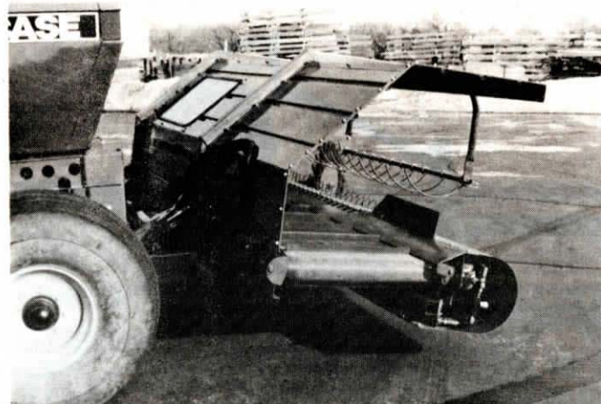
Seven ft. wide hay pickup lifts windrow and places it on 24-in. wide belt. Belt carries windrow to the side of the tractor.
