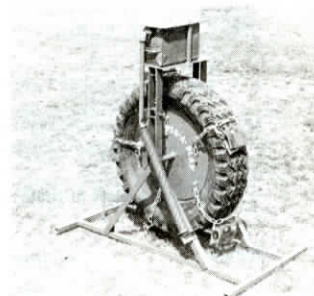
Oiler operates independent of the rotating wheel.
