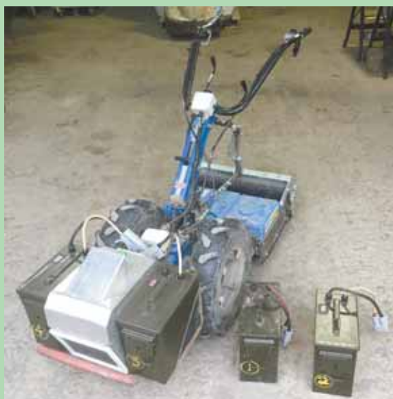
Two-wheeled, walk-behind tractor is operated by a DC motor off a Motrec utility cart. It’s powered by a pair of battery packs off a Chevrolet Volt.
