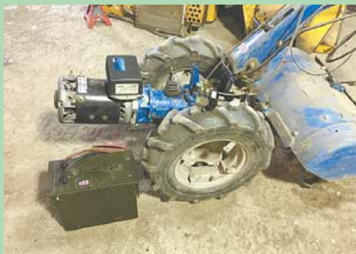
Allaway removed the clutch and fabricated an adaptor plate and shaft coupler to mate the DC motor to the BCS transmission’s input shaft and bell housing.
