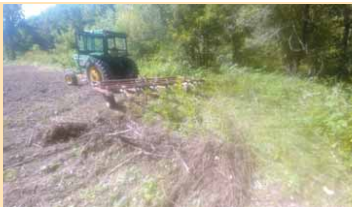
He removed the shovels from all the shanks, then added 2 shanks between the center 3 ones. That created 10-in. spacing to catch smaller sticks.
