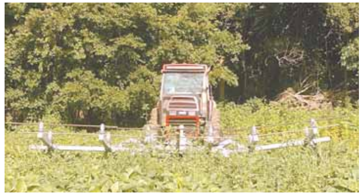
Boom mounts on front of most tractors and is powered by a rear-mounted, pto-driven generator.
