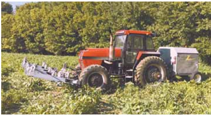
Electric-powered Weed Zapper kills weeds by using an electric charge to explode weed cells from tip to root.
