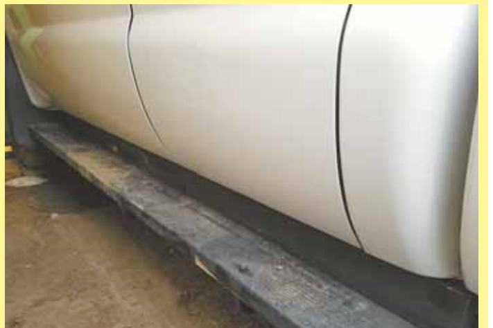
Gary Swensen mounted wooden running boards made from 2 by 8's on his Ford F-250 pickup. "They aren't fancy but they work fine," he says.
