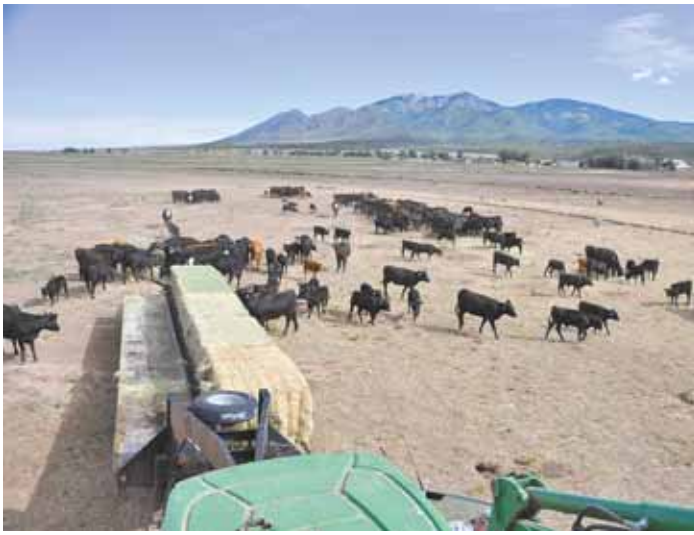
Chain pulls pushing arm that moves bales to the rear. Arm gradually pushes bales off one side of platform, then returns to front and swings over to push bales off other side.
