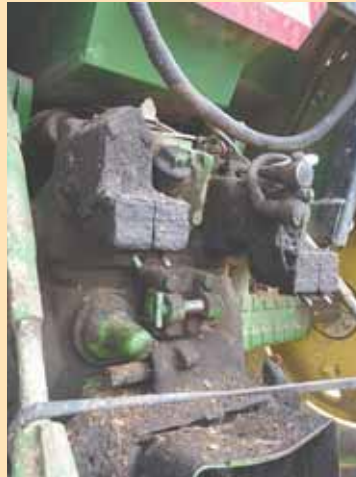
Kit converts leaky hydraulic outlets on older Deere tractors to ISO couplers that thread into an insert and connect under pressure.
