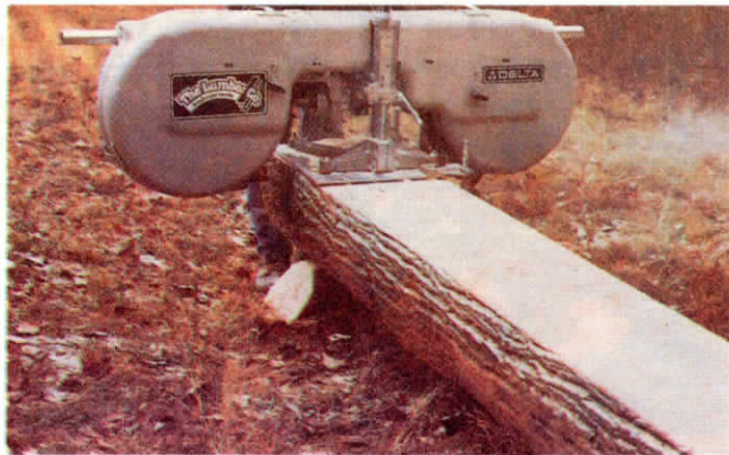
The Lumber Company converts to vertical band saw for edging, re-sawing.
