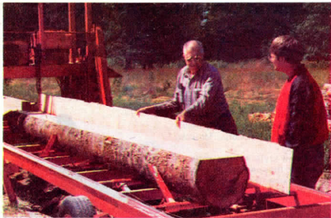
All-hydraulic sawmill handles logs up to 36 in. dia. and 20 ft. long.
