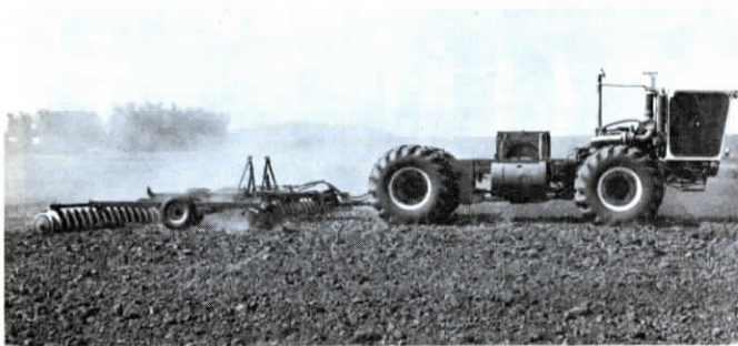
Telescoping frame of the "Hauler" extends 5 ft. to accommodate a 600 bu. grain box, converting it from tractor to truck.
