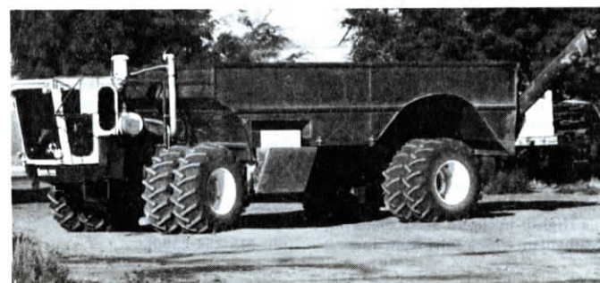
Note unloading auger at rear which allows driver to empty the 600 bu. box right from the cab.
