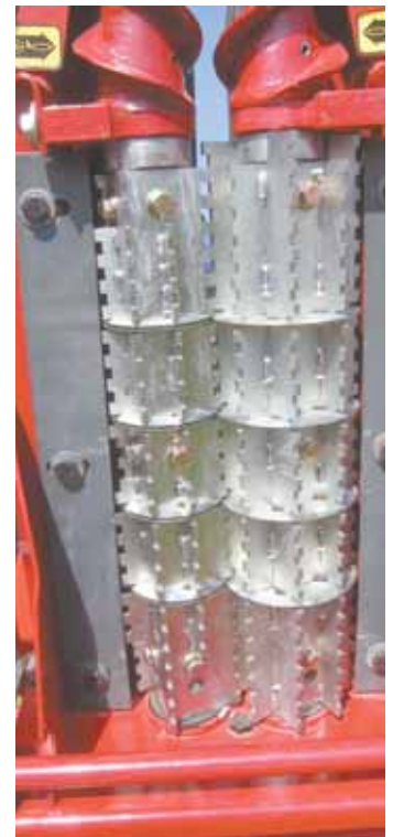
Vence Tudo header comes with 2 overlapping stalk rolls per row, one smaller than the other. Rolls run at different speeds to open pith of stalk from top to bottom.
