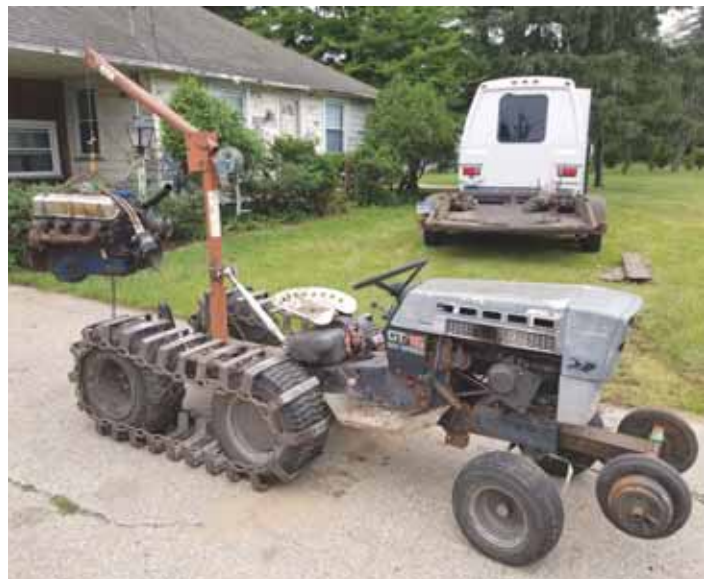
Mike Hodgson’s Sears garden tractor will go just about anywhere, thanks to its home-made half-tracks. A manually-operated boom bolts on between tracks.
