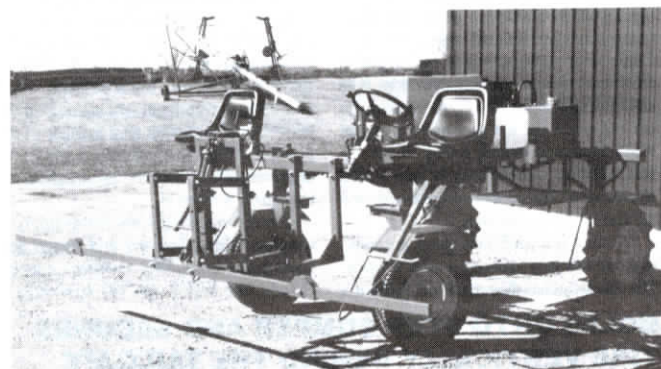
Little Boy II has hydrostatic drive and is powered by a 9 hp electric start engine.
