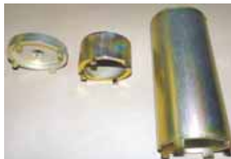
Eric Rego and his dad machine service tools and parts kits for Oliver tractors, including spanner sockets (left) and alignment tools.
