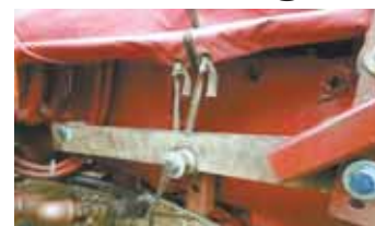
Gary Swensen bolted a 1/2-in. thick steel bar onto the frame of his Farmall 450 loader tractor to add strength for heavy loader work.
