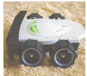
Roving robot reduces eggs laid on ground by 20 percent by keeping chickens moving.
