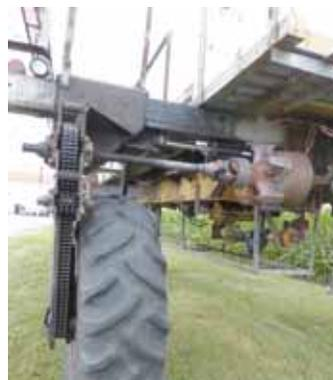
Back end of spreader was replaced with the rear end from a Chevy truck and the mechanical final drive system from a Deere combine.
