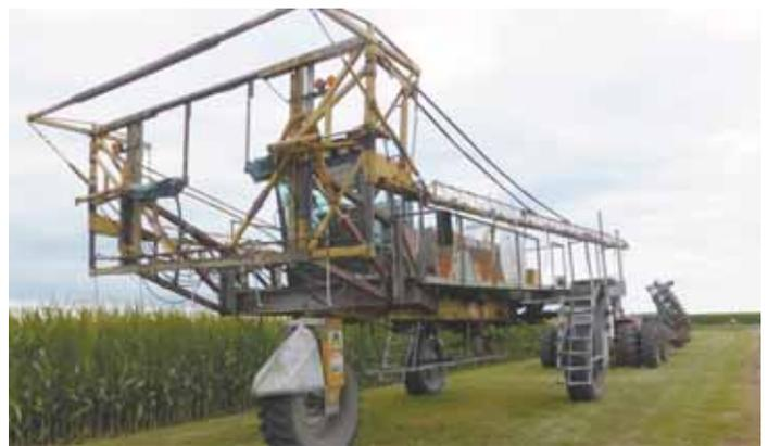
Howard Ewen built this adjustable row-width, High Boy crop sprayer by converting a worn out Big A fertilizer spreader. “Sitting up high on it is like riding in a cloud,” he says.
