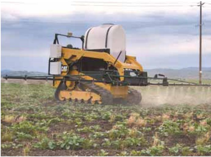
Dave and Bill Farb developed their own autosteer technology using this driverless Cat Track Loader, which can “communicate” with any pull-type or 3-pt. implement.
