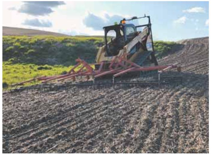
Self-driving tractor handles everything from disking to cultivating, harrowing, seeding, and spraying. Software pairs machine’s control system with GPS guidance.
