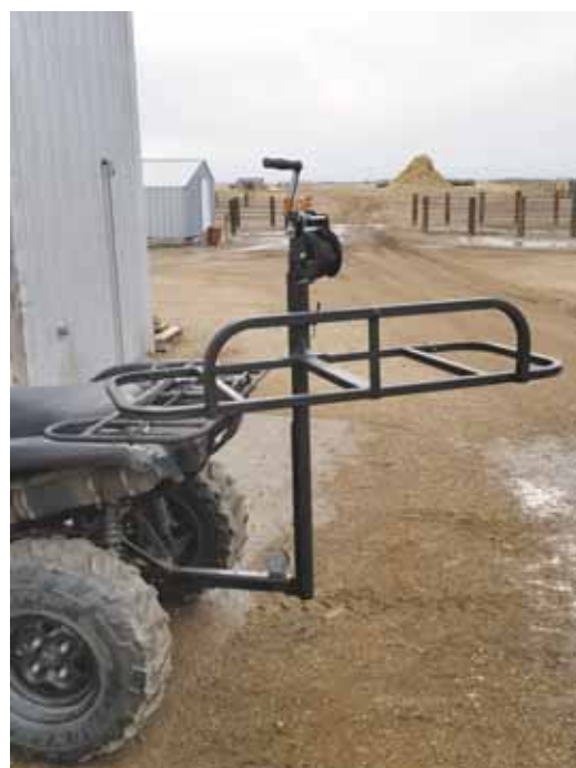
Lift is also available with a hand-cranked winch.
