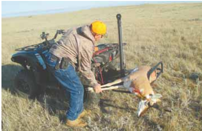
“Swivel lift” game carrier for ATV’s and pickups is designed to lift the load and then swivel it 180 degrees in either direction.
