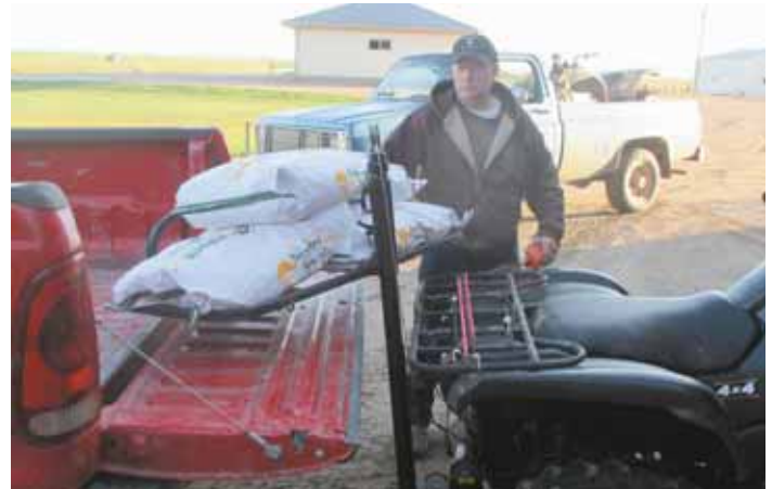
Unit comes with an electric winch with handheld remote, a vertical lift pole with a pulley on top that’s free to swivel, and a carrier basket that’s hinged at both ends.
