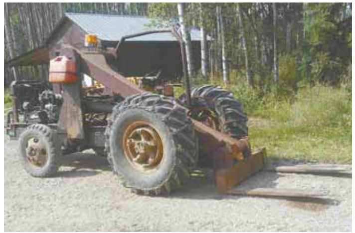
“It’s low to the ground so it’s very stable. And with the big tires on front I’m not likely to get stuck,” says Allan Isaac about his home-built forklift tractor.
