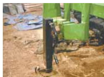
Truck pintle hooks bolted onto skid loader quick-tach plate make it easier to maneuver drill into a tight parking spot (upper left). Driver matches pintle hooks up with horizontal pins on drill’s 2-pt. hitch (above). Four truck landing gear jacks make it easy to raise entire drill.
