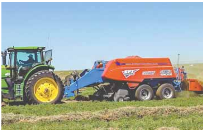
Jason Grady and his father Mike cut apart 2 balers and put them back together behind a big baler pickup to combine them into a single machine.
