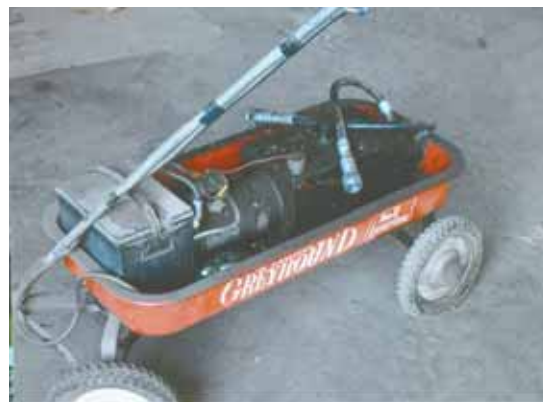
To raise drill row units off the ground, Mills placed an electro/hydraulic unit on a kids wagon and hooked a 12-volt battery up to it. Hoses connect to drill’s lift cylinders.
