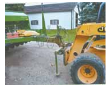
Truck pintle hooks bolted onto skid loader quick-tach plate make it easier to maneuver drill into a tight parking spot (upper left). Driver matches pintle hooks up with horizontal pins on drill’s 2-pt. hitch (above). Four truck landing gear jacks make it easy to raise entire drill.
