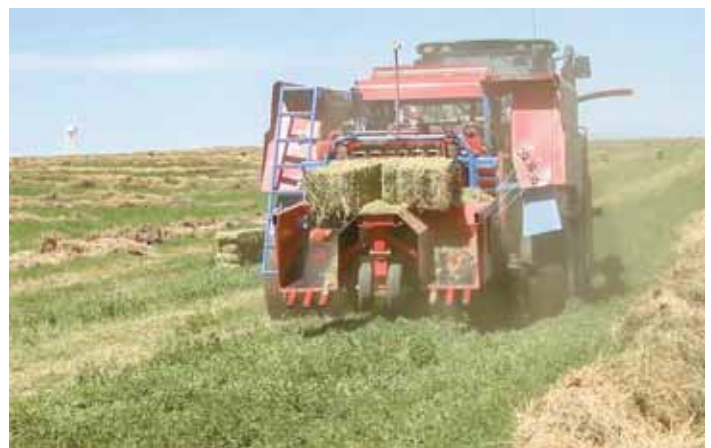
Double baler can produce about 85 percent as much tonnage per hour as a big baler, and 2 to 3 times more bales than the fastest small bale balers on the market.
