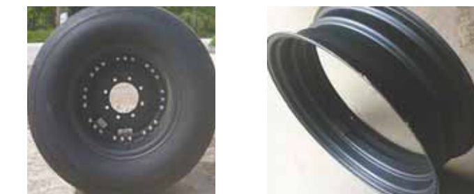
Hey Machinery installs aircraft tires on different size ag wheels with varying bolt patterns. They also make several different kinds of rims, including metric sizes.
