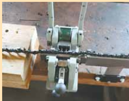
Mose Troyer's chain-breaking tool simplifies making saw chains from bulk roll stock.
