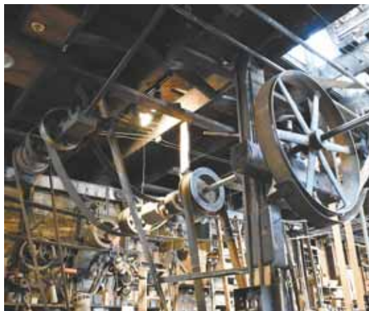
Factory's original line shaft and all the belt-driven equipment it operates are still in working condition.
