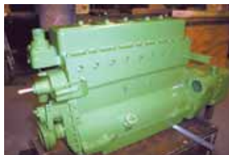
Dossdall cast every part for the 1/2-scale engine, building it in 2 halves which he bolted together.
