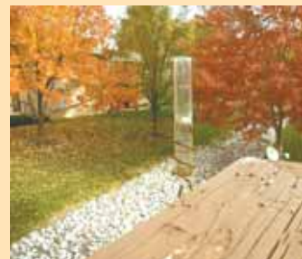
Styrofoam ball floats to top of water inside gauge, making it easy to see water level.
