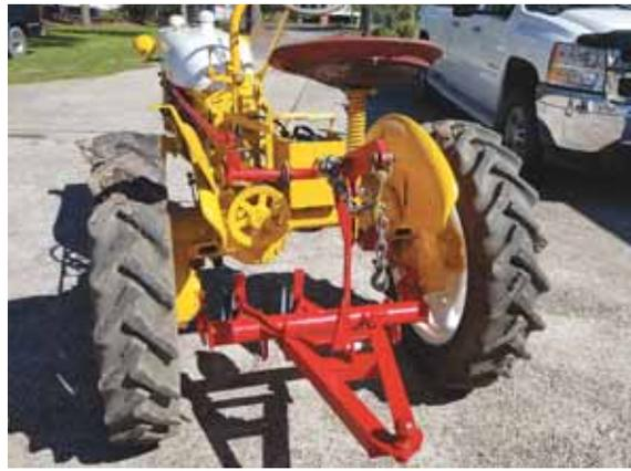
Triangle-shaped ball hitch makes it easy to hook up trailers and move them around. "I lower the hitch to the ground, lift the trailer, and then automatically unhook at the new location," says LeBlanc.
