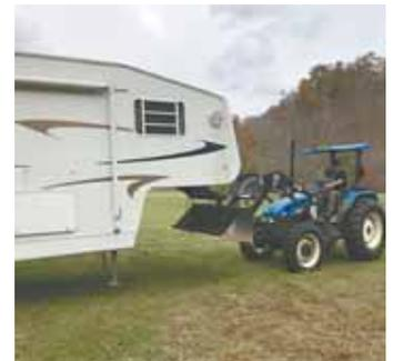
Short steel pipe welded on top of bucket forms a "cup" to lift camper's king pin.
