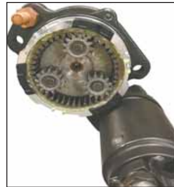
Planetary gears in starter are encased in the center, resulting in more torque and a faster engine start.
