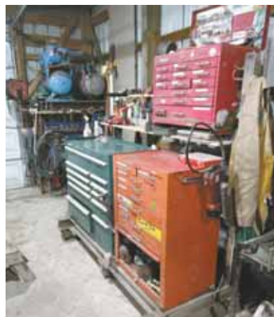
Welded-together I-beam frame holds 3 toolboxes of different sizes together to keep tools more organized.
