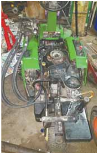
Heron mounted the power steering pump off a big truck toward back of mower and attached a pulley on top of it. He also attached a pulley to the flywheel on top of mower's engine.
