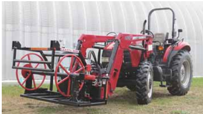
Combination wire winder and post puller for skid loaders and loader tractors lets one person roll up multiple wires at a time, and also pull up fence posts.
