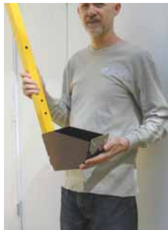
Bottom Digger is also used to dig and pull out loose dirt. "It pulls through the trench like a backhoe bucket on a stick," says Greg Baka.
