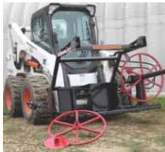
An orbit motor rotates a shaft to wind up the wire, which is contained inside a pair of big metal wheels (left). Post puller consists of 2 large thick steel plates opened or closed by a hydraulic cylinder.
