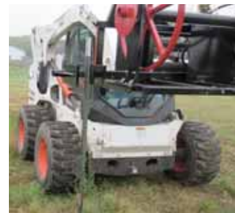
An orbit motor rotates a shaft to wind up the wire, which is contained inside a pair of big metal wheels (left). Post puller consists of 2 large thick steel plates opened or closed by a hydraulic cylinder.
