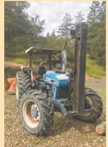
Front-mounted splitter is built on an 8 by 6-in. I-beam that folds up vertically out of the way when not in use.
