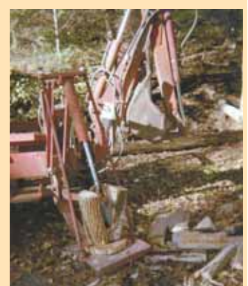
When Ray Horan needed a log splitter, he decided to convert one of the "outriggers" on his Ditch Witch.
