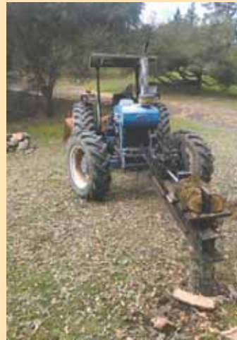
Front-mounted splitter is built on an 8 by 6-in. I-beam that folds up vertically out of the way when not in use.
