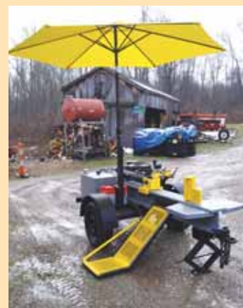
"It's built so strong that it'll never twist or bend," says James Queen about his hydraulic-operated log splitter. He can quickly set up a 10-ft. umbrella over it.
