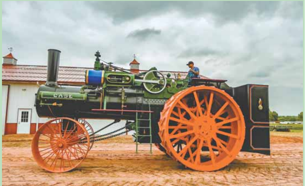
About 8,000 people from around the world saw Kory Anderson's home-built Case 150 steam engine in action last September at a South Dakota show. At 150 hp., it has been described as the world's largest steam engine. Only 9 were built between 1905 and 1907, and none survived.
