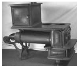
This patented "twisted hay burner" used removable, spring-operated cylindrical magazines to feed hay into the stove. A supply of packed cylinders would be kept at the ready.
