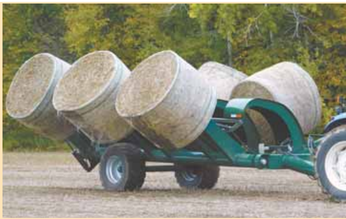
Three sets of hydraulically-operated bale spears extend and retract to grab bales in the row, with no need to crisscross the field.
