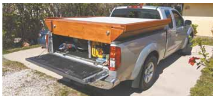
Home-built wooden "tonneau topper" extends above and outside the box on Brad Kane's Nissan pickup. He uses it to carry two 6-ft. wide work tables.
