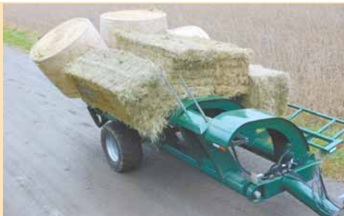
Machine can handle a combination of big square and round bales on the same load.
