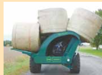
Hydraulic cylinders push speared bales up and over rack.
