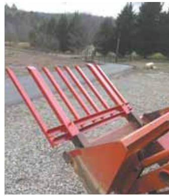
Bucket-mounted brush hauler fits over tines on loader bucket. Brush saw is welded to a forklift fork that attaches to bucket floor. Mathis tilts bucket as he drives saw into roots.
