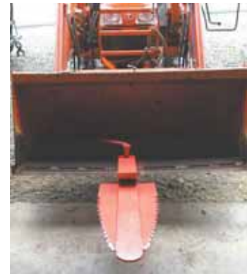
Bucket-mounted brush hauler fits over tines on loader bucket. Brush saw is welded to a forklift fork that attaches to bucket floor. Mathis tilts bucket as he drives saw into roots.
