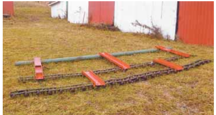
Lindsay Gillis needed to smooth out his pasture, so he built this 14-ft. wide by 6 1/2-ft. drag out of pipe and old Caterpillar dozer rails.
