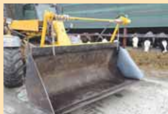
Two ropes drop down from horizontal winch and attach to cow's feet. As winch brings cow closer, operator tilts bucket upward.
