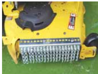
Photo shows how redesigned chain guard can be mounted on a curved chute. Bottom photo shows straight model on a Kubota riding mower.
