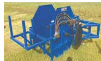
Hydraulic-powered grain bag roller can be mounted on a skid loader, front-end loader, or trailer.
