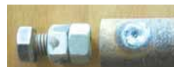
To attach pipes to wheels, Buelke welded a 5/8-in. nut inside the 1-in. dia. pipes so he can turn them onto the tractor bolts. To weld nut in place, he drills a small hole in side of pipe just above the end.
