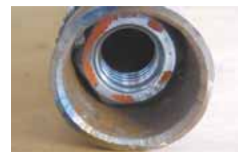
To attach pipes to wheels, Buelke welded a 5/8-in. nut inside the 1-in. dia. pipes so he can turn them onto the tractor bolts. To weld nut in place, he drills a small hole in side of pipe just above the end.
