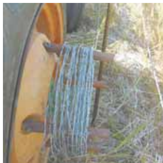
Four 10-in. long pipes attach to studs on tractor’s rear wheel hub. To wind up fence wire, Buelke jacks up wheel and puts tractor’s transmission in gear.
