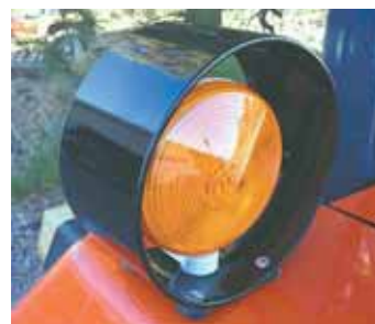
LightGuard is designed to protect fender-mounted stud lights. It consists of a 6-in. dia., 3-in. deep powder-coated aluminum ring with 4 rubber “feet”. A slot in one side makes mounting easy.
