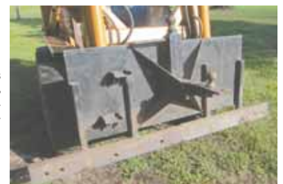
Modified quick-tach plate is equipped with a 2-in. ball hitch, gooseneck hitch, steps, and a 6-ft. long, 5-in. high grader blade.
