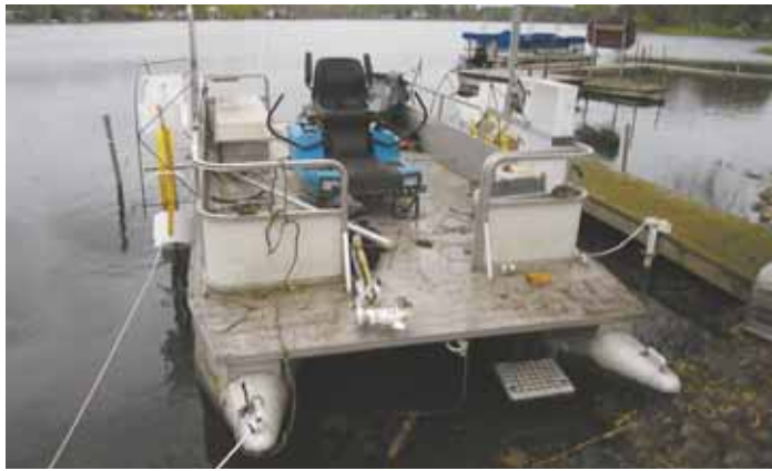
Roy Philpot's one-of-a-kind pontoon is driven by a pair of 4-ft. dia. paddle wheels about halfway back on the boat. They're powered by an old zero-turn riding mower.
