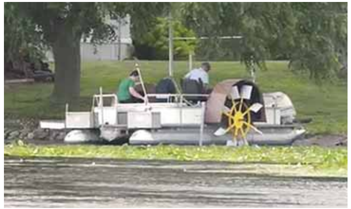
After removing mower's wheels and deck, he extended the drive axles out to both sides of boat. Each paddle wheel contains eight 12-in. sq. paddles cut out of plastic barrels.
