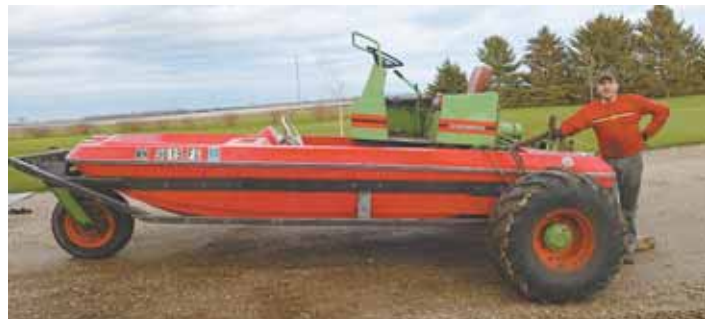
Ken Heley's amphibious "Rowatonna" paddleboat is powered by the engine off an Owatonna swather, and also uses swather's hydrostatic drive wheels and operator's platform.
